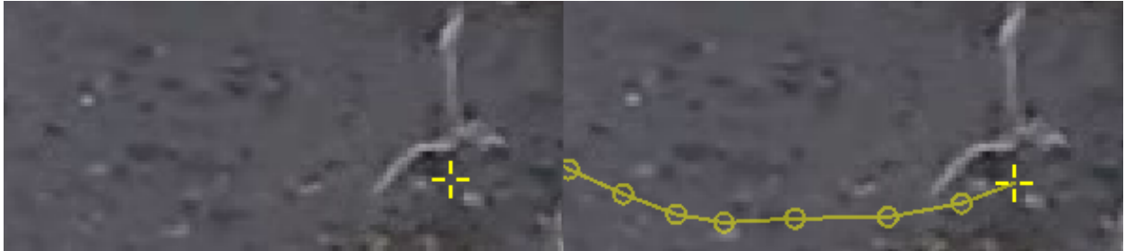
Fig. 11: The same marker in normal mode (left) and in tracking mode (right). The track always displays all previous positions connected with a line, when they are from two consecutive images.
